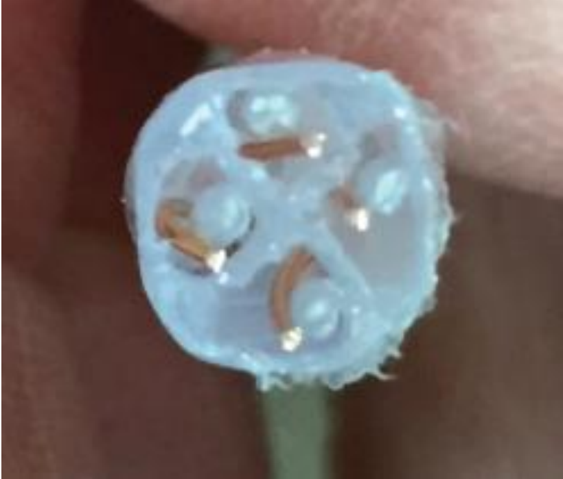
AIR spaced CONDUCTORS with FEP TEFLON THREAD SPACERS.
